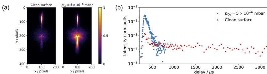
Fig. 7 (a) Comparison of the CO scattering VMI on the clean surface (no oxygen in the chamber) and  $p_{O_2} = 5 \times 10^{-6}$  mbar at  $T_s = 600$  K. (b) shows the corresponding CO scattering kinetic trace in (a); data are selected within a 20-degree sector below the center and signals are normalized to the incident beam intensity.
