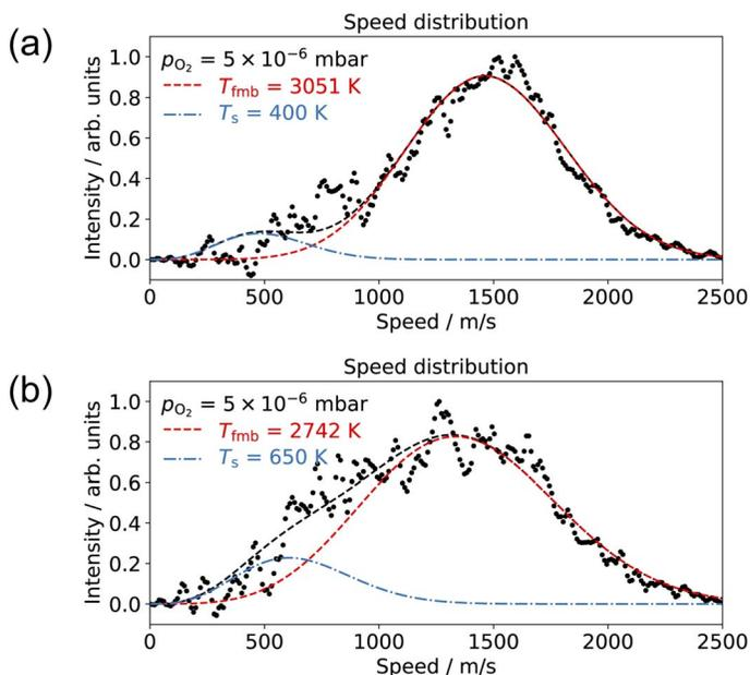
Fig. 8 Comparison of the CO<sub>2</sub> speed distribution for CO oxidation with 10% CO/He molecular beam and  $p_{\text{O}_2} = 5 \times 10^{-6}$  mbar in the scattering chamber at surface temperatures of (a) 400 K and (b) 650 K.
