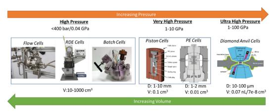
Fig. 9 Range of high-pressure electrochemical reactors with varying volume and pressure levels.
