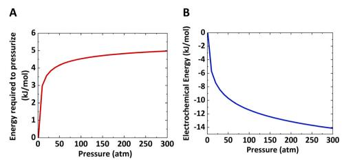
Fig. 2 Thermodynamic energy requirements: (A) energy required to pressurize a reactor as a function of pressure assuming isentropic expansion of an ideal gas. (B) Electrochemical energy reduction for any redox reaction as a function of pressure.
