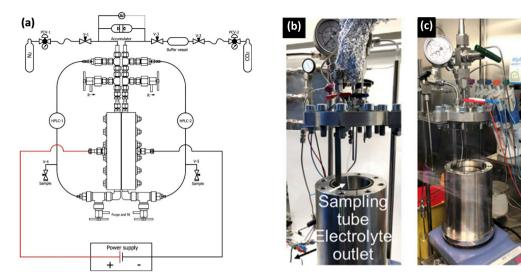
Fig. 12 Examples of autoclave setups developed for high-pressure electrochemical studies. (a) A schematic of a continuous-flow high-pressure setup for electrochemical reduction reaction, Adapted from Ramdin et al. 5 Copyright 2019 American Chemical Society. Photos of batch autoclave reactors placed in (b) the fume hood and (c) the Ar glovebox for electrochemical synthesis of ammonia. Adapted from Li et al.<sup>69</sup> Copyright 2022 The Author(s). Published by Elsevier Inc.
