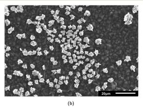
Fig. 3 SEM images of electrodeposited Nb/BDD-Ag with (a) homogeneous and (b) heterogeneous growth patterns.
