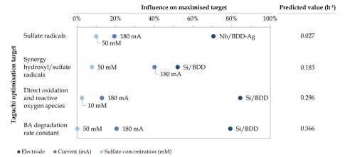
Fig. 8 Influence of the optimal experimental conditions (i.e., electrode type, current applied, and initial sulfate concentration) on the selected Taguchi optimisation targets, that is, aiming to maximise the degradation via sulfate radicals, sulfate/hydroxyl synergistic effect, direct oxidation and ROS as well as the overall BA degradation rate constant. Predicted contributions ( $h^{-1}$ ) under the optimal conditions are also provided.
