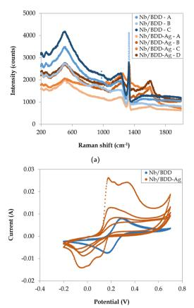
(b) Fig. 4 (a) Raman spectra at 4 different locations (A, B, C, and D) and (b) CV experiments (4 cycles) for Nb/BDD and Nb/BDD-Ag electrodes.
