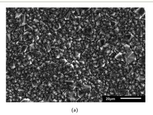
Fig. 1 SEM images of commercial (a) Nb/BDD and (b) Si/BDD electrodes.
