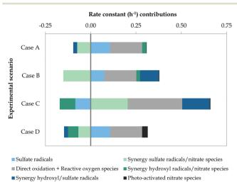
6 Rate constant contributions (h<sup>-1</sup>) of the degradation mechanisms involved in the removal of BA through scenarios A to D The operating parameters of each experimental scenario are depicted in Table 2
