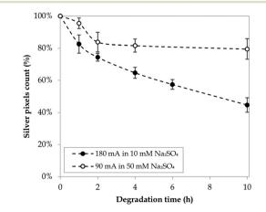
Stability tests of the Nb/BDD-Ag electrode surface.
