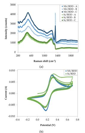
Fig. 2 (a) Raman spectra at 3 different locations (A, B, and C) and (b) CV experiments (4 cycles) for Nb/BDD and Si/BDD electrodes.
