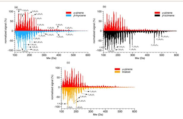
Fig. 4 SOA mass spectra. High-resolution mass spectra of SOA formed from photooxidation of  $\alpha$ -pinene compared to the mass spectra of SOA formed from (a)  $\beta$ -myrcene, (b)  $\beta$ -ocimene, and (c) linalool in an OFR. Spectra from both ESI (+) and ESI (-) modes were combined, and the x-axis represents the neutral mass. The signal for each peak is scaled to the normalized intensity
