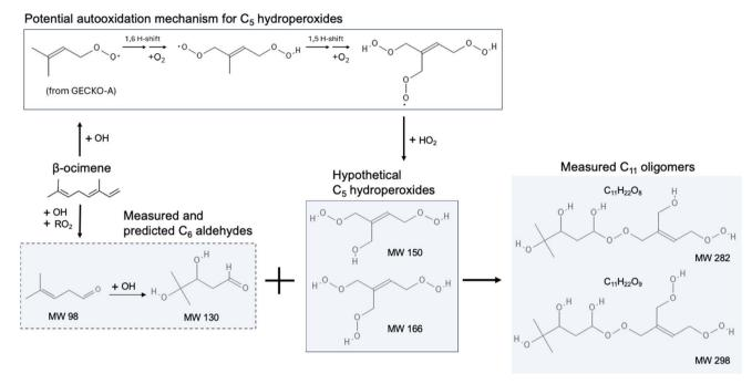
Fig. 5 One possible reaction mechanism that could generate  $C_{11}$  oligomers from  $\beta$ -ocimene oxidation. The  $C_{6}$  aldehydes in the shaded box with a dashed outline are predicted by GECKO-A modeling and have matching neutral masses in the ESI HRMS spectrum
