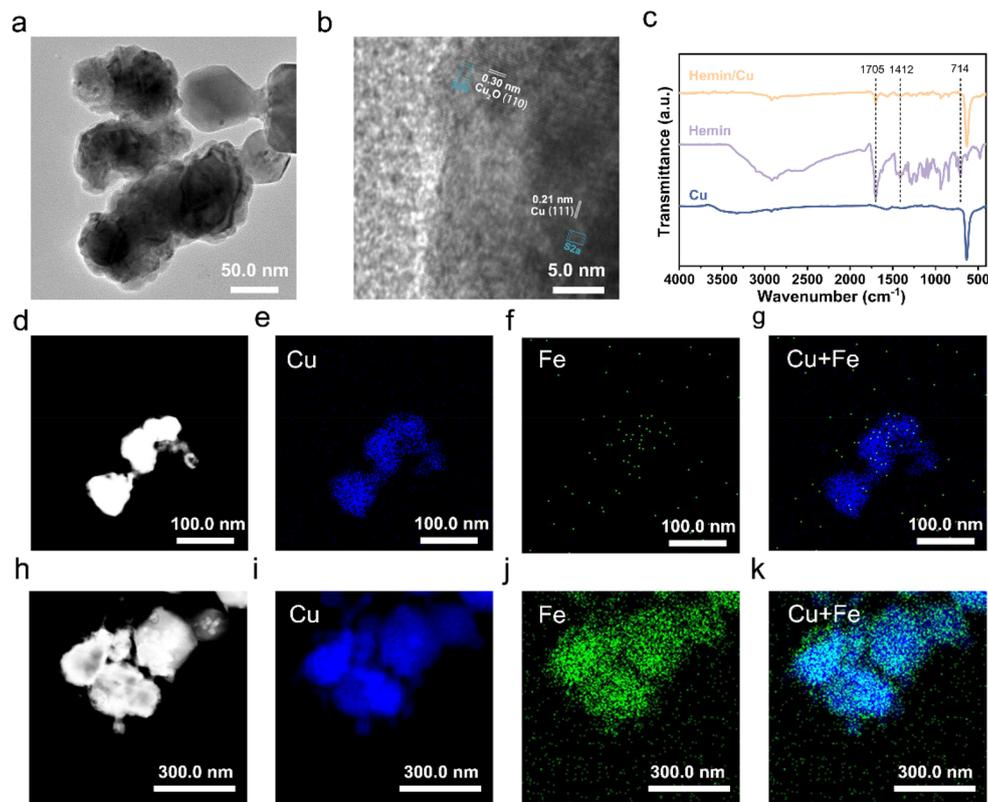
**Fig. 1** Characterization of the electrocatalysts. (a) TEM and (b) HRTEM images of Cu NPs. (c) FTIR spectra of the as-synthesized Cu, hemin, and hemin/Cu-6. HAADF-STEM images and the corresponding EDS elemental maps of (d–g) Cu NPs and (h–k) hemin/Cu-6.
