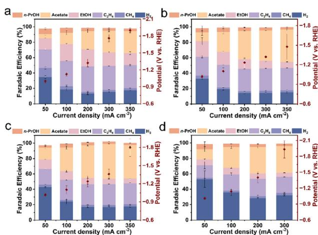
**Fig. 2** CO reduction performances of Cu NPs and hemin/Cu with different mass ratios in a flow cell system. FEs and potentials measured for the electroreduction of CO on (a) Cu NPs, (b) hemin/Cu-20, (c) hemin/Cu-6, and (d) hemin/Cu-1.
