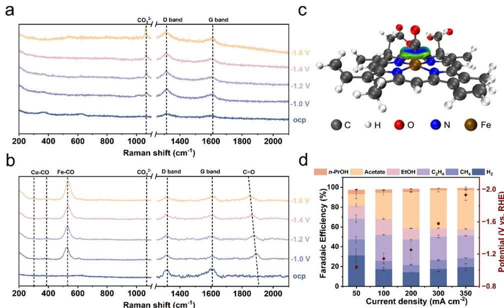
**Fig. 4** Mechanistic investigations and verification of universality. Operando Raman spectra of (a) the Cu NP electrode and (b) the hemin/Cu-6 electrode during the CORR at different applied potentials vs. RHE in 1 M KHCO<sub>3</sub>. (c) IGMH analysis of the optimized geometries of heme and the CO complex (isosurface = 0.04 a.u., visualized by VMD and the Multiwfn program). (d) Product distribution at different current densities over CoPc/Cu NPs-6.
