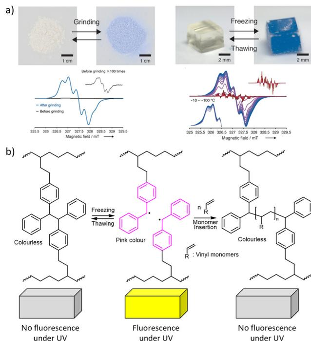
**Fig. 8** Mechanochromism from chain fracture to macroradicals that absorb visible light. (a) Top: DABBF-linked polymers change colour after grinding their powders or freezing their hydrogels. Bottom: The ESR spectra confirming the formation of radicals. Adapted from ref. 32 with permission. (b) Polymerisation of acrylate solutes initiated by TASN radicals during freeze–thaw cycles. See Fig. 2 for the chemical structures.
