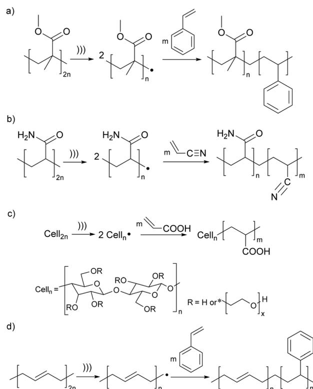
**Fig. 4** Examples of polymerisation of monomers initiated by mechanochemically-generated macroradicals from: (a) acrylates; (b) polyacrylamide; (c) cellulose; (d) butadiene. ))) signifies ultrasound; radical chain terminations are not shown. Adapted from ref. 54, 55, 57 and 58.
