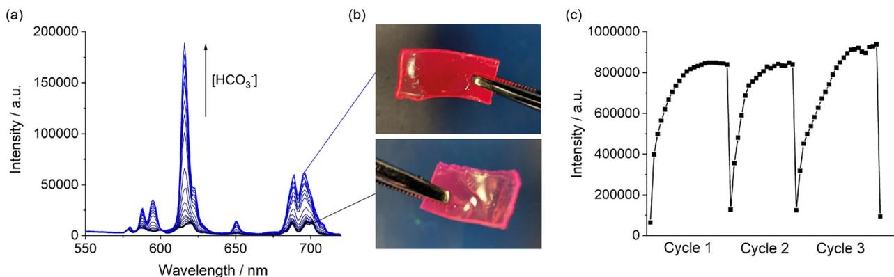
Fig. 3 (a) Emission titration of  $[\text{Eu.1}]^+$  loaded particles with bicarbonate. (b) Photos of hydrogels containing  $[\text{Eu.1}]^+$  loaded particles under UV-light, showing the visual increase in red emission intensity upon 15 minute incubation with bicarbonate. (c) Reversible increase in emission of the hydrogel upon three repeat sensing cycles, involving incubation with 30 mM bicarbonate, followed by washing in buffered aqueous solution.
