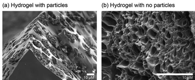
Fig. 2 Scanning electron microscopy (SEM) images of (a) hydrogels containing  $[\text{Eu.1}]^+$  loaded particles embedded in the pores of the hydrogel, and (b) hydrogels lacking particles showing unoccupied pores.
