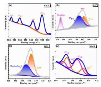
Fig. 3 X-ray photoelectron spectroscopy spectra of  $C_3M_1OS$ : high resolution-XPS spectra of (a) Cu 2p, (b) S 2p, (c) O 1s, and (d) Mn 2p.
