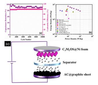
Fig. 7 Electrochemical characteristics of the  $C_3M_1OS//AC$  asymmetric device: (a) recyclability test at 10 A g<sup>-1</sup> and the corresponding Coulombic efficiency, (b) Ragone plot at several current loads in comparison with previously reported devices in the literature, and (c) schematic diagram of the developed C<sub>3</sub>M<sub>1</sub>OS//AC asymmetric device
