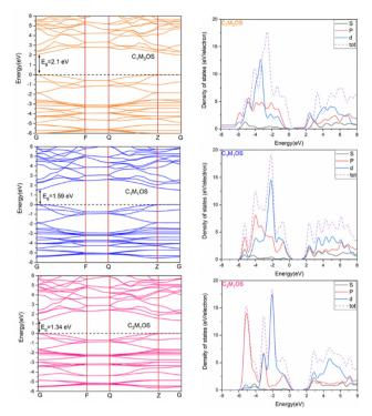
Fig. 9 Electronic band structure and projected DOS of  $C_1M_3OS$ ,  $C_1M_1OS$ , and  $C_3M_1OS$ . The Fermi level is defined as the top of the valence band represented by the dashed line at 0 eV.
