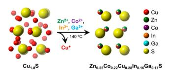
**Fig. 2** Figure visually showing the formation of  $(Zn_{0.25}Co_{0.22}Cu_{0.28}Ln_{0.16}-Ca_{0.11})$ S HE metal sulfide synthesis *via* simultaneous multication exchange. Copyright permission from American Chemical Society, used from ref. 65.
