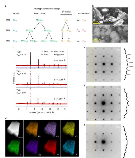
Fig. 9 (a) Composition design of HEO cathodes with variations of TM ions, (b) SEM images of as-synthesized TM6, (c) synchrotron XRD patterns and refined lattice parameters of the as-prepared HEOs, (d) HAADF-STEM EDX mapping of elemental distribution in a particle cluster of TM6. Scale bar, 300 nm. (e)-(g) TEM ED patterns measured on TM2 (e), TM4 (f) and TM6 (g) along the [100] zone axis. Copyright permission from Nature materials, used from ref. 146.
