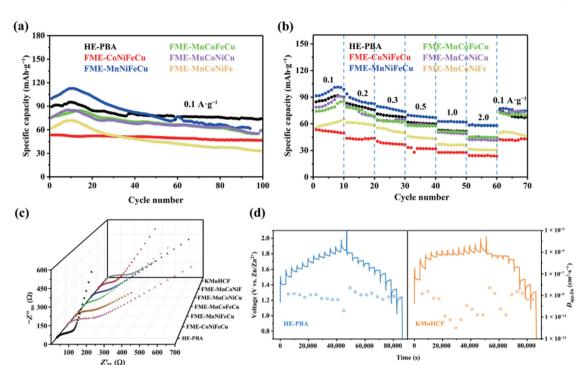
Fig. 19 Electrochemical performance of HE-PBA as ZIB: (a) cycling capability at  $0.1 \, \mathrm{A} \, \mathrm{g}^{-1}$ , (b) rate performance, (c) Nyquist plots of different electrodes, (d) GITT curves and corresponding  $\mathrm{Z} \, \mathrm{n}^{2+}$  diffusion coefficients of HE-PBA and KMnHCF during charge/discharge process, respectively. Copyright permission from Nano research, used from ref. 192.
