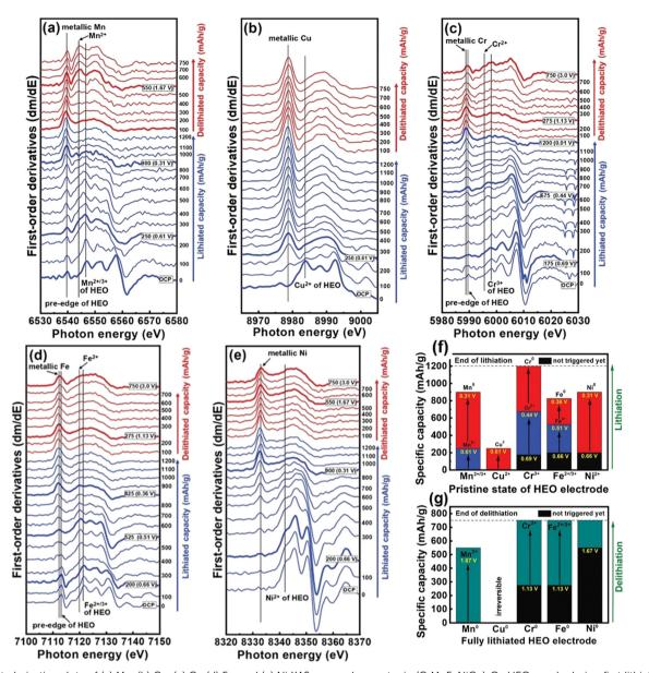
Fig. 8 First-derivative plots of (a) Mn, (b) Cu, (c) Cr, (d) Fe, and (e) Ni XAS operando spectra in (CrMnFeNiCu)<sub>3</sub>O<sub>4</sub> HEO anode during first lithiation and delithiation cycle at 150 mA g<sup>-1</sup> current density. (f)-(g) Capacity contribution of all constituent elements in HEO electrode during first lithiation and delithiation cycle. Copyright permission from Wiley, used from ref. 49
