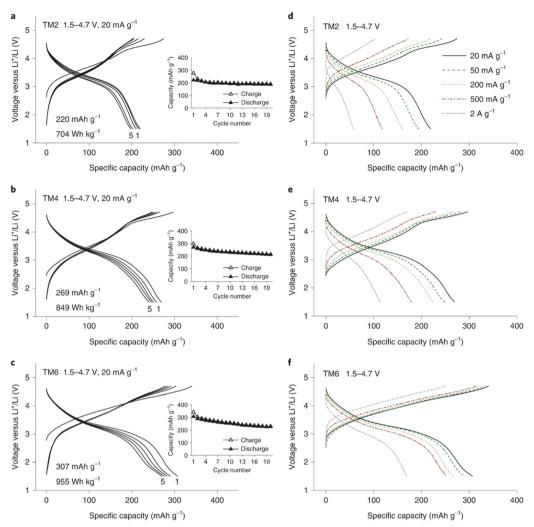
Fig. 10 Voltage curves of TM2 (a), TM4 (b) and TM6 (c) within the potential scope of 1.5-4.7 V at 20 mA  $g^{-1}$  current density (insets show the capacity retention plots), rate performance of TM2 (d), TM4 (e) and TM6 (f) exhibiting the 1st voltage curves between 1.5 and 4.7 V at 20, 50, 200, 500 and 2000 mA  $g^{-1}$ . Copyright permission from Nature materials, used from ref. 146.
