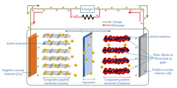
Fig. 1 Model of the battery with all components depicting the process of charging and discharging using the direction of flow of electrons. The arrows and electrons in red depict the discharging process, whereas those in green depict the charging process. The electrons flow *via* the connecting wires, and the positive ions diffuse to either electrode (positive or negative) depending on the process of charging and discharging *via* the electrolyte.
