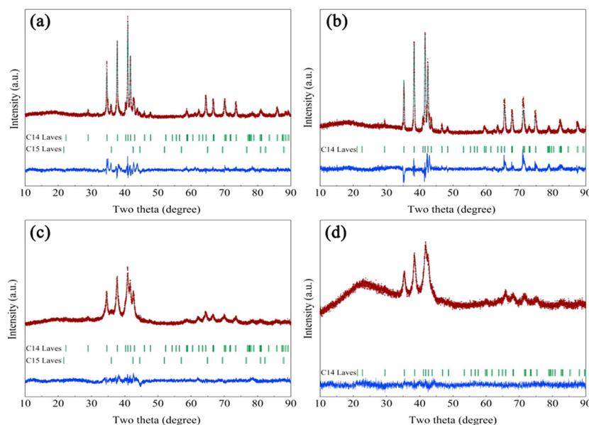
Fig. 1 Rietveld refinements of the XRD patterns for (a) Zr<sub>2</sub>V<sub>2</sub>CrNi, (b) Zr<sub>2</sub>VFeCrNi, (c) Zr<sub>2</sub>MgV<sub>2</sub>CrNi and (d) Zr<sub>2</sub>MgVFeCrNi high-entropy alloys.
