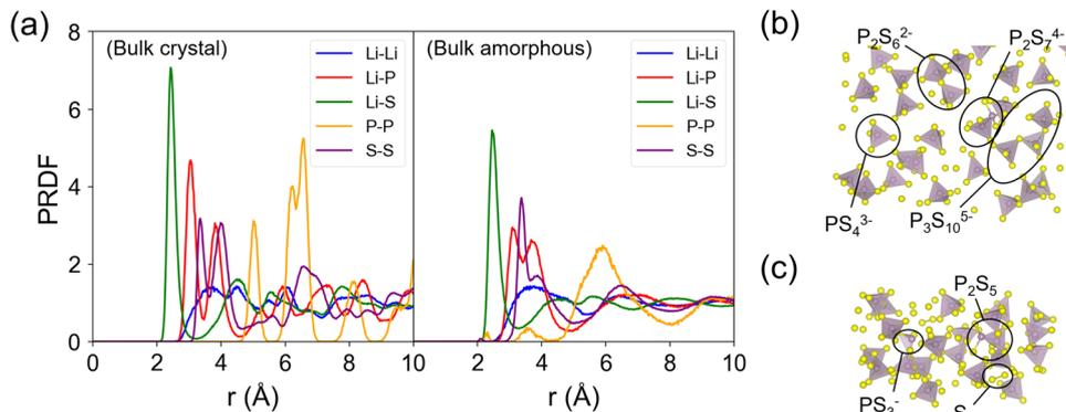
Fig. 4 (a) Partial radial distribution function (PRDF) plots of crystalline and amorphous  $\beta$ -LPS from MD simulations. The two PRDF subplots share the same vertical axis. (b) and (c) Representative local P–S structures in the amorphous  $\beta$ -LPS. Distinct host framework polyanion units are labeled; polyanion units are searched by incremental sweep of atom–atom distance and finding the minimum distance that results in polyhedral unit formation for all P atoms.
