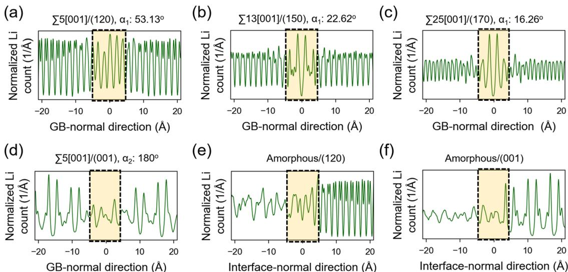
Fig. 7 Projected Li concentration profiles around the grain boundary (GB) and amorphous/crystal interface regions: (a)  $\Sigma 5[001]/(120)$  tilt GB, (b)  $\Sigma 13[001]/(150)$  tilt GB, (c)  $\Sigma 25[001]/(170)$  tilt GB, (d)  $\Sigma 5[001]/(001)$  twist GB, (e) amorphous/(120) interface, and (f) amorphous/(001) interface. Enclosed regions highlight the GB region. A Gaussian kernel smoothing procedure is performed with a covariance factor of  $1.0 \times 10^{-4}$ .
