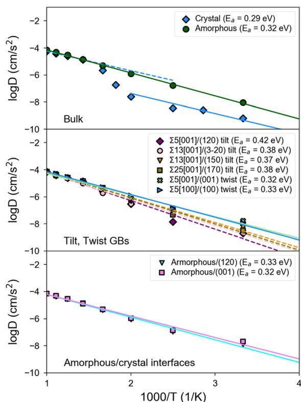
Fig. 5 Arrhenius plot of the log of the  $\text{Li}^+$  diffusivity ( $\log D$ ) versus inverse temperature ( $1000/T$ ) in (top) bulk crystal and amorphous  $\beta$ -LPS; (middle) GBs and (bottom) amorphous/bulk interfaces of  $\beta$ -LPS. The  $E_{a,\text{bulk}}$  value is fitted using the Arrhenius slope at the low temperature regime.
