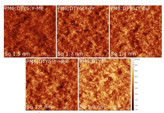
Fig. 4 AFM height images ( $2.5 \times 2.5 \, \mu m^2$ ) of the active layers of the ternary and binary blends prepared on glass/ITO/PEDOT:PSS substrates. The corresponding phase images are shown in Fig. S12 (ESI†).
