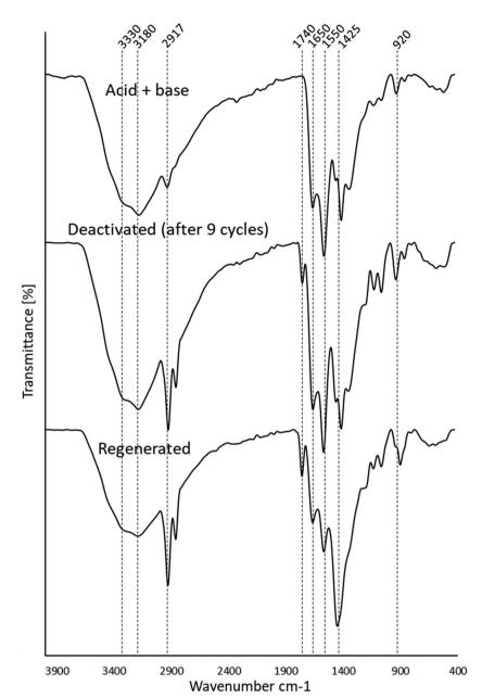
Fig. 8 Stacked FTIR spectra of the basified catalyst, the deactivated and regenerated catalysts
