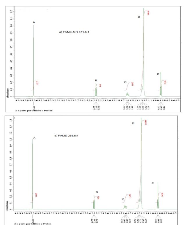
Fig. 2 A typical <sup>1</sup>H NMR spectrum of sample (a) FAME-MR 571.5:1 and (b) FAME-MR 285.5:1 with labelling of the major peaks, reaction conditions: reaction temperature 65 °C, 2 h and over 1.5 g of basified PANF fibrous solid catalyst.
