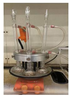
Chart 1 Transesterification reaction under water-cooled reflux in Radley Carousel reactor.
