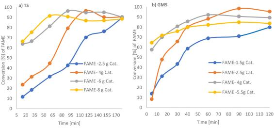
Fig. 4 GC-FID analysis for the conversion of TS and GMS to FAME as a function of solid base PANF catalyst loading. (a) TS to methyl ester for a molar ratio of methanol to TS 285.5:1, total vol. 108.95; and (b) GMS to FAME for a molar ratio of methanol to GMS 115.1:1, total vol. 107.74 mL, at 65 °C.
