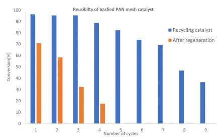
Fig. 6 GC-FID analysis for conversion of tristearin (TS) to FAME as a function of the number of cycles. Reaction conditions: 65 °C, 3 h, 3 g of catalyst, Molar ratio of methanol to TS was 274:1, volume = 27.34 mL.
