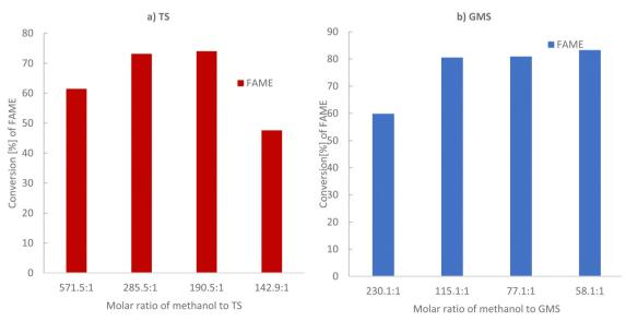
Fig. 3 GC-FID analysis for conversion of triglyceride tristearin (TS) and monoglyceride glycerol monostearate (GMS) to (FAME) as a function of their molar ratio. (a) Tristearin (TS) conversion and (b) GMS conversion. Reaction conditions: 65 °C, 2 h, 1.5 g of solid base PANF catalyst.
