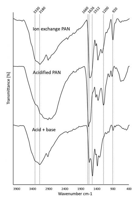
Fig. 7 Stacked FTIR spectra of the ion exchange PANF, the ion exchange PAN in its acidified and basified forms.
