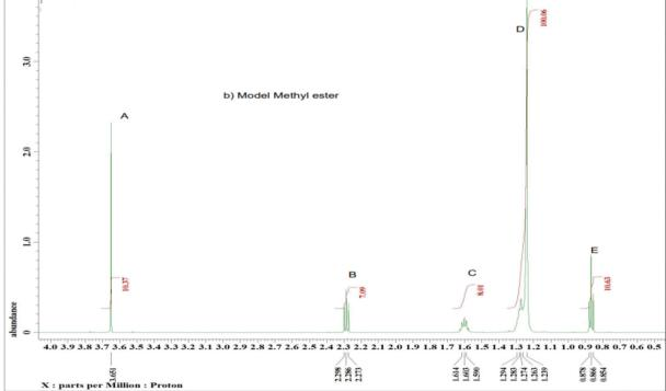
Fig. 1 A typical <sup>1</sup>H NMR spectrum of the model compounds (a) tristearin and (b) methyl stearate with labelling of the major peaks.
