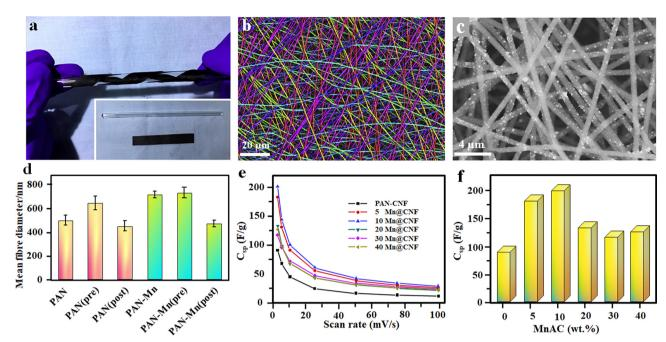
Fig. 5 (a) Flexible free standing composite film of PAN-20 wt% MnACAC after carbonisation. (b and c) FE-SEM image of pure PAN fibers (colorized to distinguish orientation) and PAN with 40 Mn@CNF, respectively. (d) Mean diameter of different spun fibers. (e) Variation of specific capacitance with scan rate. (f) Specific capacitances of the all-fiber supercapacitors with different MnACAC concentrations at 2.5 mV s<sup>-1</sup>. Reproduced from ref. 59 with permission from Elsevier, copyright 2018.
