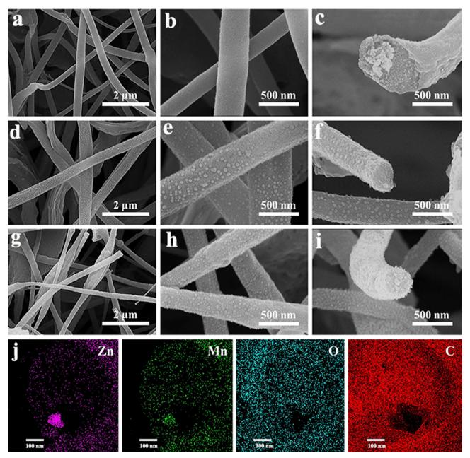
Fig. 16 FE-SEM micrographs of Zn-Mn bimetallic oxides with varying ZnAc/MnAc ratio: (a) and (b) ZMTS1 (ZnAc:MnAc = 1:3); (d) and (e) ZMTS2 (ZnAc: MnAc = 2:2); (g) and (h) ZMTS3 (ZnAc:MnAc = 3:1) at different magnification. (c), (f) and (i) Corresponding cross-sectional images of ZMTS1, ZMTS2 and ZMTS3, respectively. (j) The elemental mapping of different elements such as Zn, Mn, O and C present in the CNFs (ZMTS3). Reproduced from ref. 130 with permission from Wiley, copyright 2022.
