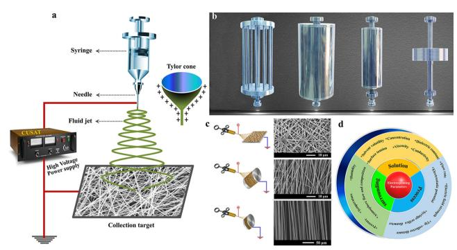
Fig. 2 (a) Basic instrumentation. Reproduced from ref. 57 with permission from Springer, copyright 2021. (b) Different types of collectors. Reproduced from ref. 60 with permission from Springer, copyright 2016. (c) Microstructure of various alignments of fiber with different types of collectors in electrospinning. Reproduced from ref. 61 and 62 with permission from Elsevier, copyright 2015, Royal Society of Chemistry, copyright 2017. (d) Factors affecting electrospinning technique.
