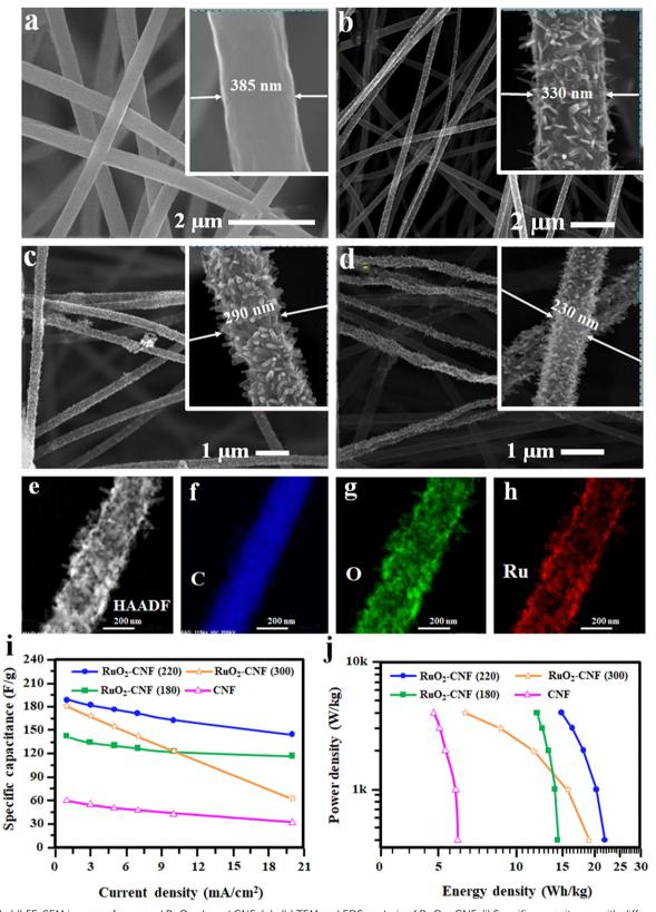
Fig. 10 (a)-(d) FE-SEM images of pure and RuO<sub>2</sub>-doped CNF. (e)-(h) TEM and EDS analysis of RuO<sub>2</sub>-CNF. (i) Specific capacitance with different current densities and (j) Ragone plot of RuO2-CNF flexible SC. Reproduced from ref. 102 with permission from American Chemical Society, copyright 2020.
