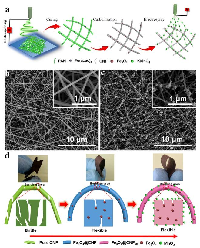
Fig. 12 (a) Schematics of flexible Fe<sub>3</sub>O<sub>4</sub>@CNFMn electrode preparation. (b and c) FE-SEM micrographs of the Fe<sub>3</sub>O<sub>4</sub>@CNF and Fe<sub>3</sub>O<sub>4</sub>@CNFMn fiber electrode respectively. (d) Photographs and mechanism of the enhanced flexibility of the Fe<sub>3</sub>O<sub>4</sub>@CNFMn electrode. Reproduced from ref. 108 with permission from Nature, copyright 2017.
