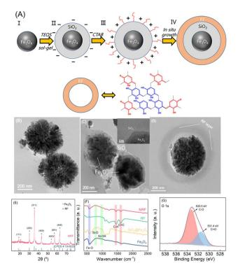
Fig. 1 (A) Schematic synthetic procedure of the magnetic resorcinol-formaldehyde photocatalysts; (B)–(D) TEM images of (B)  $Fe_3O_4$  particles, (C)  $Fe_3O_4$ @SiO<sub>2</sub> (inset: HRTEM image at the core–shell interface), and (D) MRF microspheres; (E) XRD patterns of MRF; (F) FTIR spectra of various materials; (G) high-resolution O 1s XPS spectrum of MRF.
