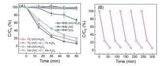
Fig. 4 (A) The removal of RhB, TC and HA via UVC/H<sub>2</sub>O<sub>2</sub>, UVC and H<sub>2</sub>O<sub>2</sub> processes in batch tests; and (B) recyclability of the process for RhB removal (RhB, TC or HA: 1 mg  $L^{-1}$ ;  $H_2O_2$ : 10  $\mu$ M).
