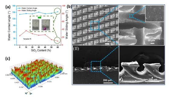
Fig. 2 (a) Dependence of the water contact and sliding angles of the stretchable PDMS elastomer formed by template TS on the SiO<sub>2</sub> content, with images of the self-cleaning test for the TS-60 sample (SiO<sub>2</sub> content: 60%) shown in the inset. (b) Top (top) and cross-sectional (bottom) views of the SEM images of TS-60. (c) Three-dimensional (3D) profile image of TS-60 for an area of 1 mm  $\times$  1 mm.
