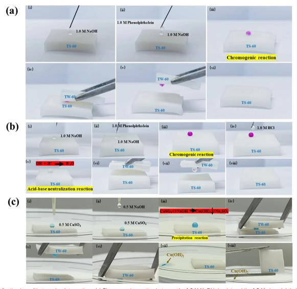
Fig. 6 Application in multi-stage droplet reactions. (a) Chromogenic reaction between the 1.0 M NaOH droplet and the 1.0 M phenolphthalein droplet, followed by transportation with TW-60 (Movie S6, ESI†). (b) Multi-stage chromogenic reactions as in (a) followed by an acid-base neutralization reaction (Movie S7, ESI†). (c) Precipitation reaction followed by transportation using TW-60 (Movie S8, ESI†).
