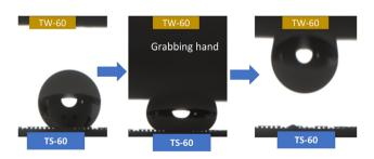
Transport of a water droplet from TS-60 to TW-60 under pressure.
