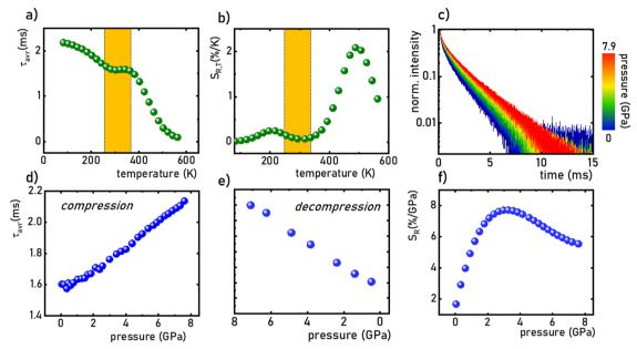
Fig. 5 The  $\tau_{avr}$  of the SrGdAlO<sub>4</sub>: 0.2%Mn<sup>4+</sup> measured as a function of temperature (a) the corresponding  $S_{R,T}$  (b); luminescence decay profile of  $SrGdAlO_4: 0.2\%Mn^{4+}$  measured as a function of pressure (c); the  $\tau_{avr}$  measured at room temperature as a function of pressure during compression (d) and decompression (e) and corresponding  $S_{R,p}$  (f).
