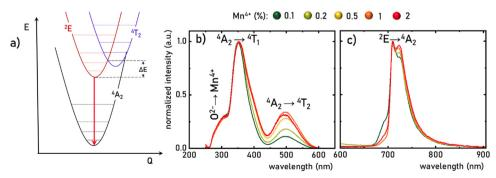
Fig. 3 Simplified configurational coordination diagram of Mn<sup>4+</sup> ions (a), the comparison of the normalized room temperature excitation spectra  $(\lambda_{em} = 710 \text{ nm})$  (b), and emission spectra  $(\lambda_{exc} = 400 \text{ nm})$  (c) of SrGdAlO<sub>4</sub>: Mn<sup>4+</sup> with different concentration of Mn<sup>4+</sup> ions.
