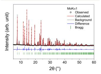
Fig. 3 Rietveld refinement of X-ray powder diffraction pattern for Li5.5-LLNZO. The experimental data are shown as black circles, the calculated pattern in red, the difference profile in blue, and calculated Bragg reflection positions in green.
