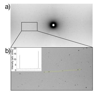
Fig. 4 (a) Representative Laue neutron diffraction image for Li5.5-LLNZO. (b) Enlarged area indicated in (a). Intensity profile through several selected reflections highlighted in yellow is shown in inset, illustrating high crystal and data quality.
