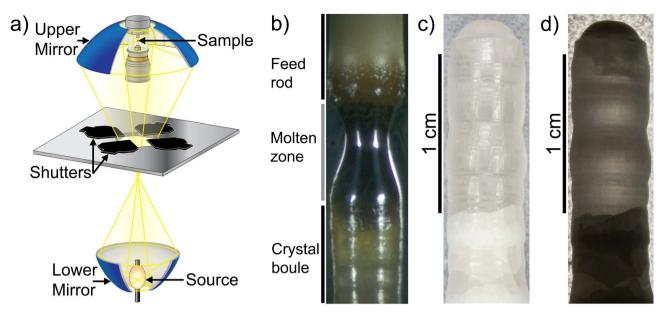
Fig. 1 (a) High-pressure single-lamp floating zone furnace setup. Figure adapted from Scientific Instruments Dresden GmbH. $^{70}$  (b) In-progress growth of Li5.5-LLNZO rod showing feed rod (top), molten zone (middle), and crystal formation (below). (c and d) Crystal boule segment synthesized with counter-rotation imaged with top lighting (c) and backlighting (d).
