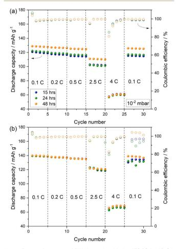
Fig. 9 Rate performance of PW electrodes dried at 170 °C for 15, 24, and 48 hours using a dynamic vacuum of  $10^{-2}$  (a) and  $10^{-3}$  mbar (b). Test conducted at 25 °C using 1 M NaPF<sub>6</sub> in diglyme electrolyte within the 2.0–4.0 V range. (1C = 140 mA g<sup>-1</sup>).
