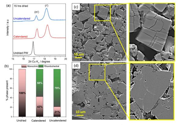
Fig. 6 (a) XRD patterns of calendared and uncalendared electrodes dried for 15 h (170  $^{\circ}$ C, 10<sup>-3</sup> mbar) relative to a pristine undried PW electrode. (b) Relative percentages of monoclinic and rhombohedral phases calculated for calendered and uncalendered electrodes. Cross-sectional SEM images of (c) uncalendered and (d) calendared pristine electrodes with zoomed areas highlighting internal crack formation.
