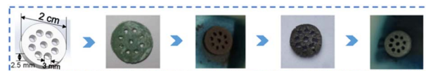
Fig. 4 Printed ceramic electrode Ti-Ni NS obtained by digital light printing technology after degreasing, sintering, and reduction, respectively [reproduced from ref. 26, with kind permission].
