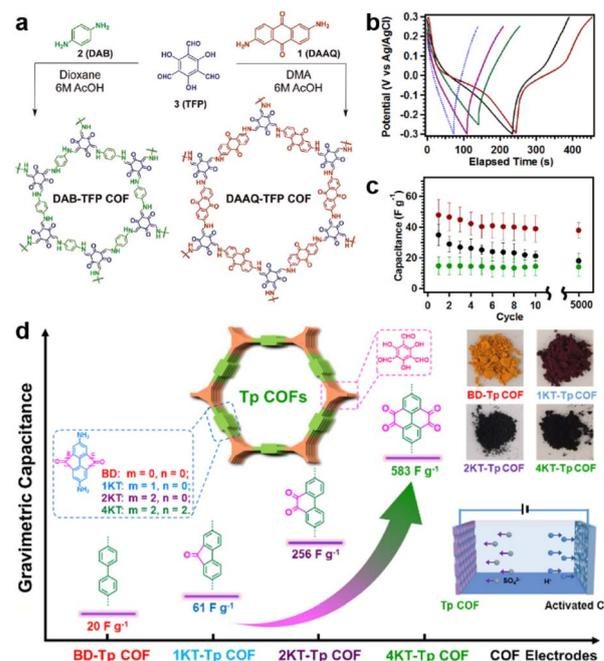
Fig. 2 (a) Synthetic routes and structures of DAAQ-TFP COF and DAB-TFP-COF. (b) GCD response and (c) average discharge capacitances at 0.1 A g<sup>-1</sup> after different cycle numbers of DAAQ-TFP COF, DAAQ monomer, and DAB-TFP COF. Reprinted from ref. 29. Copyright 2013, American Chemical Society. (d) Schematic illustration, specific capacitance, and photos of Tp-COFs with different redox groups. Reprinted from ref. 41. Copyright 2020, Chinese Chemical Society.
