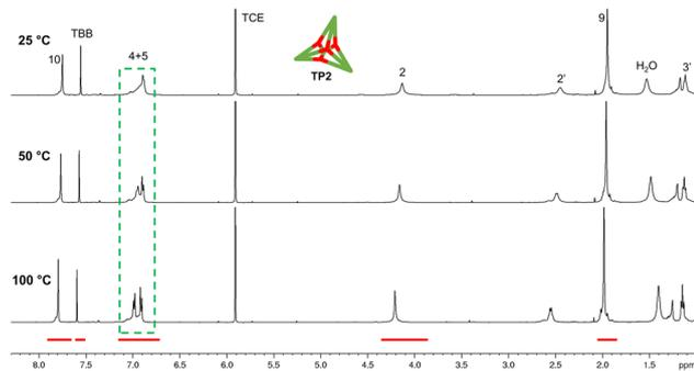
Fig. 3 qHNMR spectra (500 MHz) at different temperature of cage TP2 in TCE- $d_2$ . The green dashed rectangle highlights the appearance of a two-spin system of type AB for the aromatic protons located at C-4 and C-5 as the temperature increases. The red bars indicate the fixed integration areas for yield calculation using TBB as the internal standard. TBB = 1,3,5-tribromobenzene, TCE = 1,1,2,2-tetrachloroethane.
