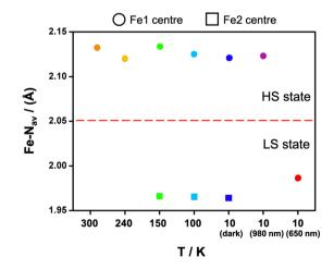
Fig. 6 Plot of the Fe- $N_{av}$  distance for 1 at 300 K (orange), 240 K (yellow), 150 K (green), 100 K (light blue), 10 K (blue), 10 K (980 nm) (purple) and 10 K (660 nm) (red). Circles represent the Fe1 centre and squares the Fe2 centre.
