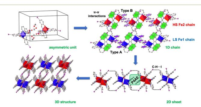
Fig. 3 Schematic illustration of the packing from the asymmetric unit to the final supramolecular 3D structure for 1 at 150 K (blue Fe1 centres, red Fe2 centres). This figure is intended as a guide to the discussion only.
