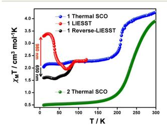
Fig. 5  $\chi_{\rm M}T$  versus T plot (recorded at 0.5 K min<sup>-1</sup>) of 1 showing the thermal behaviour in the dark without any previous light irradiation (blue), after LIESST effect at 980 nm (red) and after reverse-LIESST effect at 650 nm (black) and thermal behaviour of 2 (green).
