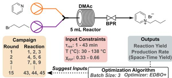
**Scheme 1** Continuous flow synthesis setup and EDBO+ workflow. Initial seed reactions were conducted within the predefined input constraints. Subsequent rounds of experiments were performed in batch sizes of three unique reactions. The outputs were used to update EDBO+ and provide the next round of suggested experiments. Initially 10 rounds of experiments were performed followed by expansion of the upper temperature constraint to 168 °C and another 5 rounds.
