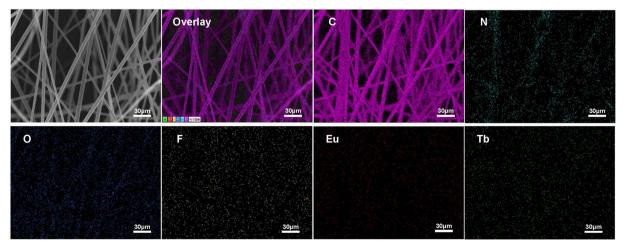
Fig. 3 Elemental mapping images of the PS-Eu<sub>1</sub>-Tb<sub>60</sub> fiber membrane.
