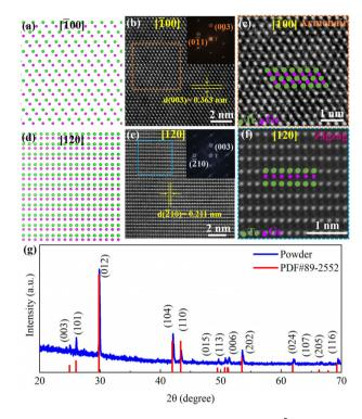
Fig. 1 (a) and (d) Simulated structure of  $\alpha$ -GeTe along  $[\bar{1}00]_R$  and  $[120]_R$ zone axes. (b) and (e) The HAADF-STEM images of  $\alpha$ -GeTe taken along [100]<sub>B</sub> and [120]<sub>B</sub> zone axes: the insets show the corresponding fast Fourier transform (FFT) patterns. (c) and (f) Zoomed-in images of the square regions in (b) and (e), respectively, for the corresponding AC and ZZ directions. (g) The powder XRD pattern of  $\alpha$ -GeTe at room temperature.
