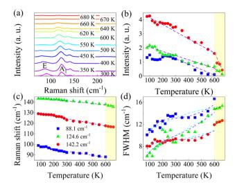
**Fig. 4** (a) Raman spectra of GeTe at different temperatures. Temperature dependence of the peak intensity (b), position (c), and FWHM (d) of the three Raman modes, where the dashed lines represent the fit results or act as a guide for the eyes.
