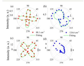
Fig. 3 (a)-(d) Polar plots of the peak intensity of E and A<sub>1</sub> modes under the polarization configurations (parallel or cross). Stars - experimental values; green curves - fit results.
