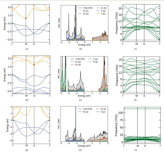
Fig. 1 Electronic band structures, density of states and phonon band structures of (a-c) Sc<sub>2</sub>CF<sub>2</sub> (first row), (d-f) Sc<sub>2</sub>CO<sub>2</sub> (second row) and (g-i) Sc<sub>2</sub>C(OH)<sub>2</sub> (third row). The y (vertical) scale of DOS plots are multiplied by 2, 2 and 5 factors for F, O and OH functional groups respectively. In the electronic band structure, the VBM and CBM are denoted by green and red points respectively.
