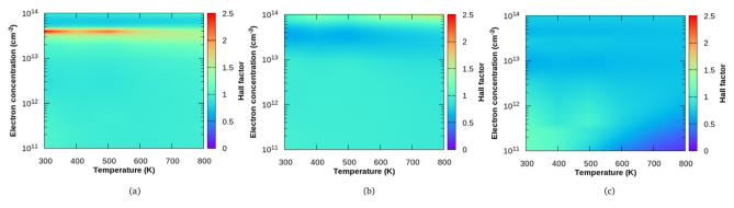
Fig. 5 Variation of the Hall factor in terms of temperature and concentration for (a) Sc<sub>2</sub>CF<sub>2</sub>, (b) Sc<sub>2</sub>CO<sub>2</sub> and (c) Sc<sub>2</sub>C(OH)<sub>2</sub>.
