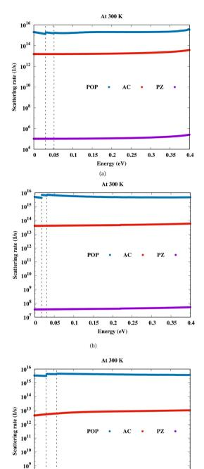
Fig. 2 Scattering rate versus energy for (a)Sc2CF2, (b)Sc2CO2 and (c) Sc<sub>2</sub>C(OH)<sub>2</sub>.
