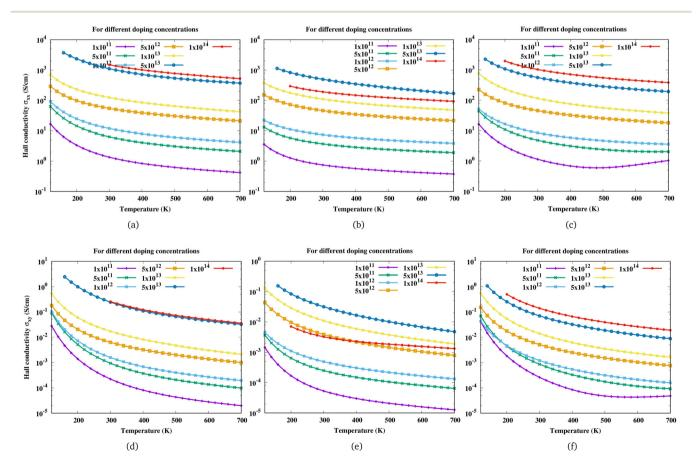
Fig. 4 Variation of Hall conductivity  $(\sigma_{xx}, \sigma_{xy})$  of (a and d)  $Sc_2CF_2$ , (b and e)  $Sc_2CO_2$ , and (c and f)  $Sc_2C(OH)_2$  with temperature at different electron concentrations. Here the first row corresponds to  $\sigma_{xx}$  and the second row to  $\sigma_{xy}$ .
