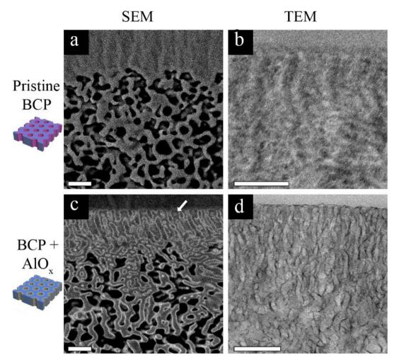
Fig. 1 Cross-sectional EM images. (a) BSE-SEM of a pristine membrane and (b) its corresponding TEM (b); (c) BSE-SEM of a membrane modified with  $AlO_x$  by SIS and ALD (the white arrow point to the top surface) and (d) its corresponding TEM. All the scale bars are 200 nm.
