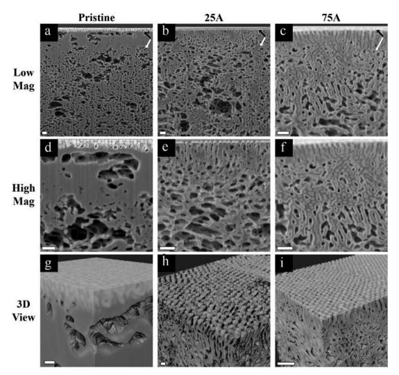
Fig. 3 (a–f) Cross-sectional SEM images and (g–i) reconstructed 3D volume of pristine membrane (a, d and g) and membrane modified with 3 cycles of  $AlO_x$  SIS and 25 (b, e and h) or 75 cycles of  $AlO_x$  ALD (c, f and i). Images d–f are higher magnifications of images a–c, respectively. The black arrows point to the highly ordered selective layer and the white arrows to the underneath supporting layer. All the scale bars are 200 nm.
