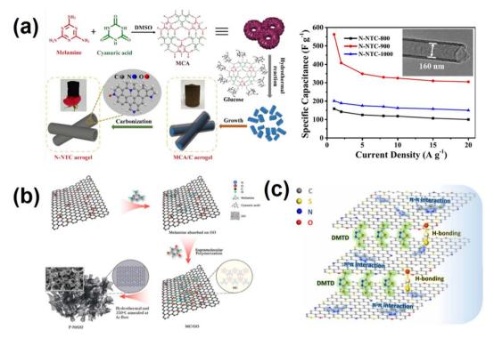
Fig. 2 (a) Schematic illustration of the synthesis and rate performance of the N-NTC aerogel.<sup>60</sup> Copyright 2021, American Chemical Society. (b) Schematic illustration of the supramolecular polymerization method for preparing P-NrGO materials.<sup>88</sup> Copyright 2018, Elsevier. (c) Schematic illustration of the interactions between GO and DMTD molecules.<sup>91</sup> Copyright 2020, Elsevier.
