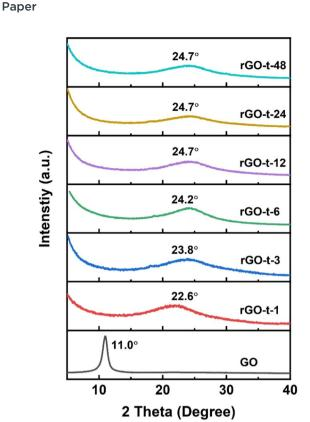
Fig. 4  $\,$  XRD patterns of GO and rGO prepared with various reduction times.
