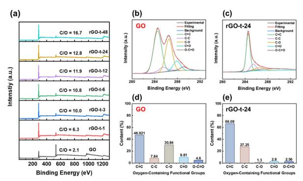
Fig. 6 (a) XPS survey spectra of GO and rGOs synthesized with various reduction times. C 1s XPS spectra of (b) GO and (c) rGO-t-24. Percentage of individual oxygenic functional groups of (d) GO and (e) rGO-t-24.
