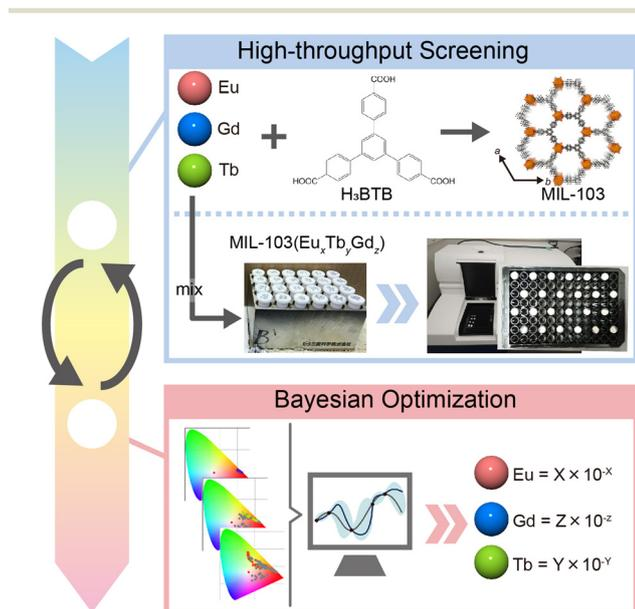
**Fig. 1** Research flow process. Data were collected by changing the stoichiometric ratio of the three lanthanide metal-salts and conducting 24 or 48 variations six times using multiple reaction vessels. Fluorescence measurements were performed using microplate readers to collect 24 spectra at a time. Based on the data, Bayesian optimization was performed to optimize the stoichiometric ratio that shows white-light emission.
