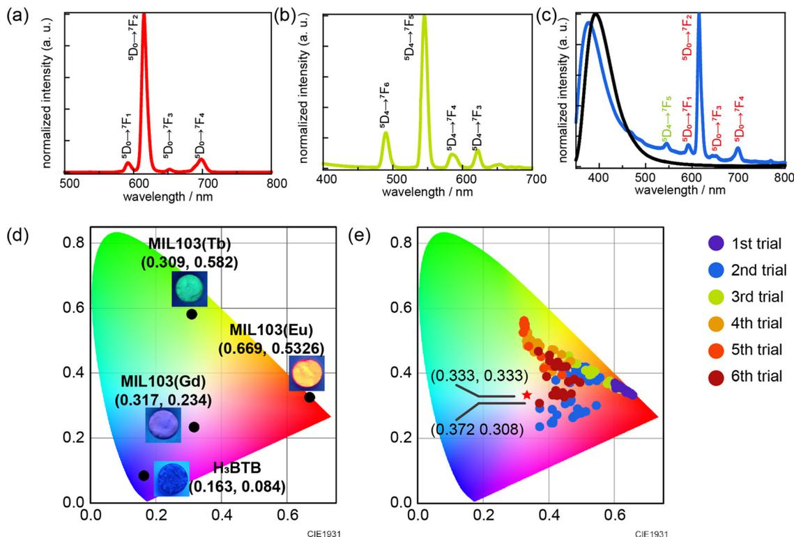
**Fig. 2** Emission spectra at an excitation wavelength of 295 nm: (a) single MIL-103(Eu), (b) single MIL-103(Tb), and (c) single MIL-103(Gd) (blue) and organic ligand H<sub>3</sub>BTB (black). (d) CIE chromaticity diagram for single MIL-103(Eu, Gd, or Tb) and organic ligand H<sub>3</sub>BTB. (e) CIE chromaticity diagram for trial experiments 1–6.
