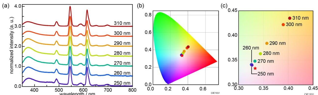
**Fig. 3** (a) Emission spectra and (b) CIE chromaticity diagram of MIL-103(Eu<sub>x</sub>Gd<sub>y</sub>Tb<sub>z</sub>; Eu =  $8.3 \times 10^{-5}$ , Tb =  $8.1 \times 10^{-3}$ , Gd =  $9.92 \times 10^{-1}$ ) at various excitation wavelengths. (c) Enlarged view of Fig. 3b.
