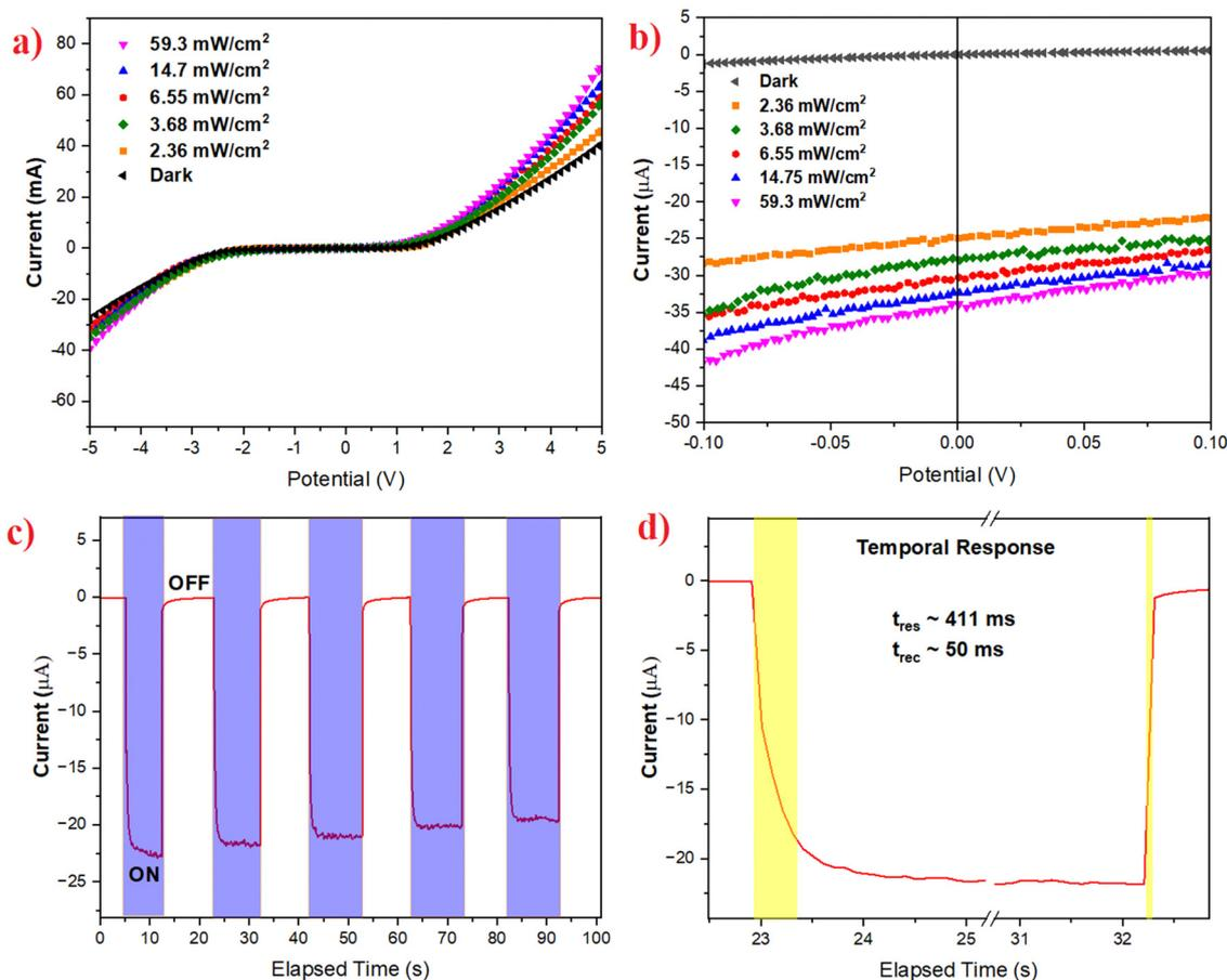
Fig. 6 Opto-electronic studies of the device fabricated using Mg : Pb-5 : 5 film.  $I$ - $V$  characteristics of the device under variation of the light intensity and voltage biasing in the range of (a)  $\pm 5$  V, and (b)  $\pm 0.1$  V. (c) The photodynamic response of the device under a solar simulator; (d) a single cycle of photodynamic response depicting the response and recovery time.
