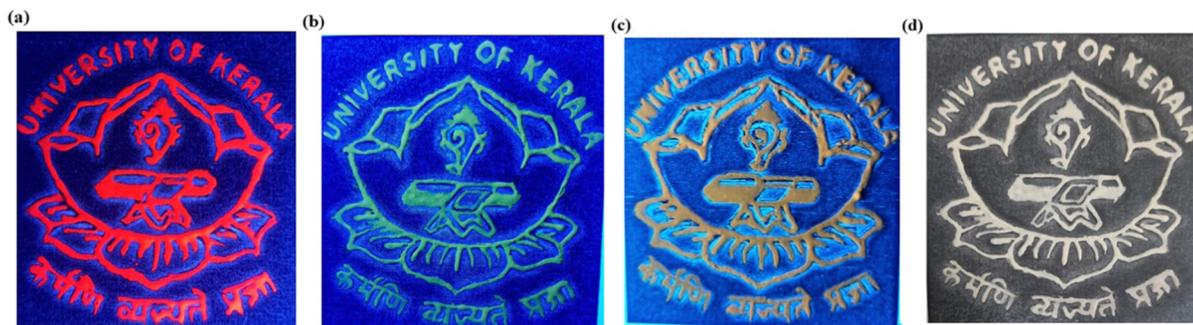
Fig. 15 Emblem of the University of Kerala illuminated under UV radiation at 365 nm using (a) SNMV:Eu<sup>3+</sup>, (b) SNMV, (c) SNMV:Sm<sup>3+</sup> phosphors, and (d) under natural light.
