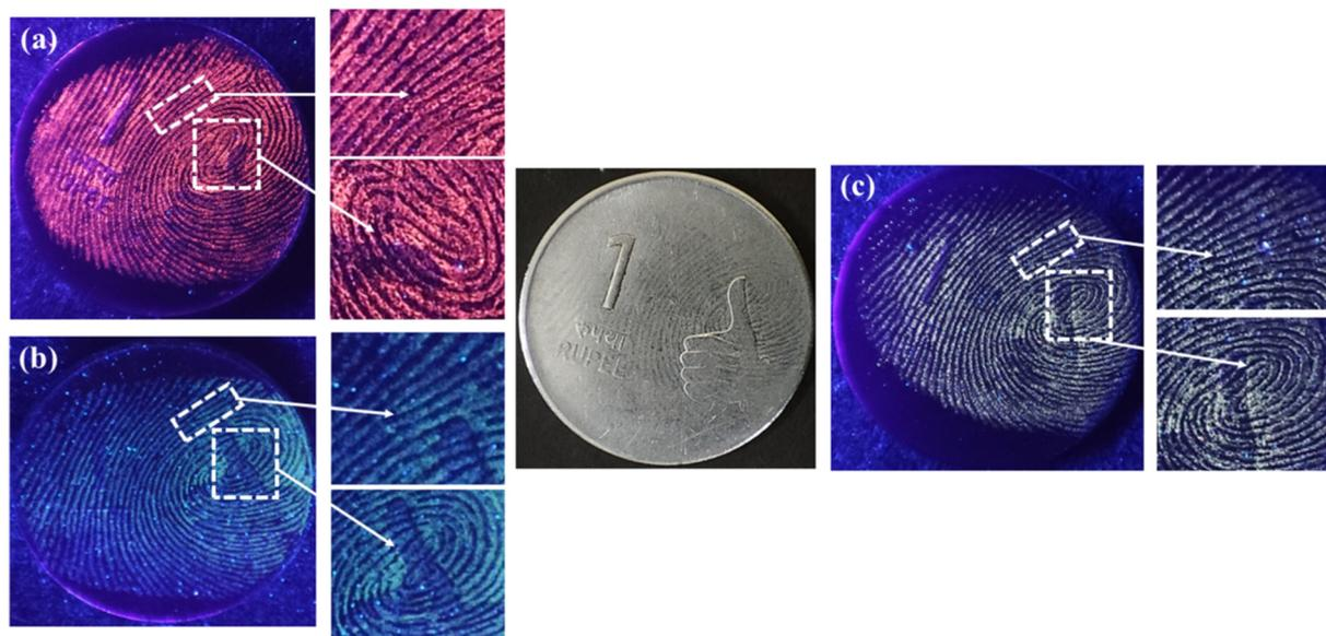
Fig. 13 Photographs of (a) SNMV:Eu<sup>3+</sup>, (b) SNMV, and (c) SNMV:Sm<sup>3+</sup> phosphor-stained LFPs on the Indian rupee coin.
