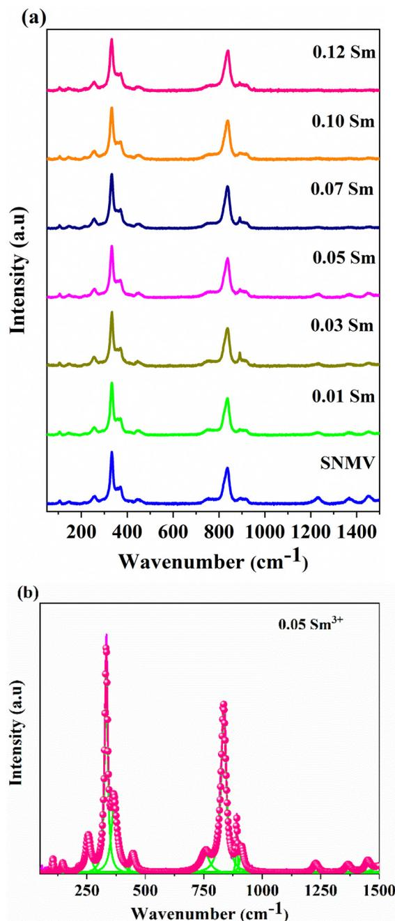
Fig. 2 (a) Raman spectra of  $\text{Sr}_2\text{NaMg}_2\text{V}_3\text{O}_{12}: x\text{Sm}^{3+}$  ( $x = 0, 0.01, 0.03, 0.05, 0.07, 0.10$  and  $0.12$ ), and (b) deconvoluted Raman spectra of SNMV:  $0.05\text{Sm}^{3+}$ .
