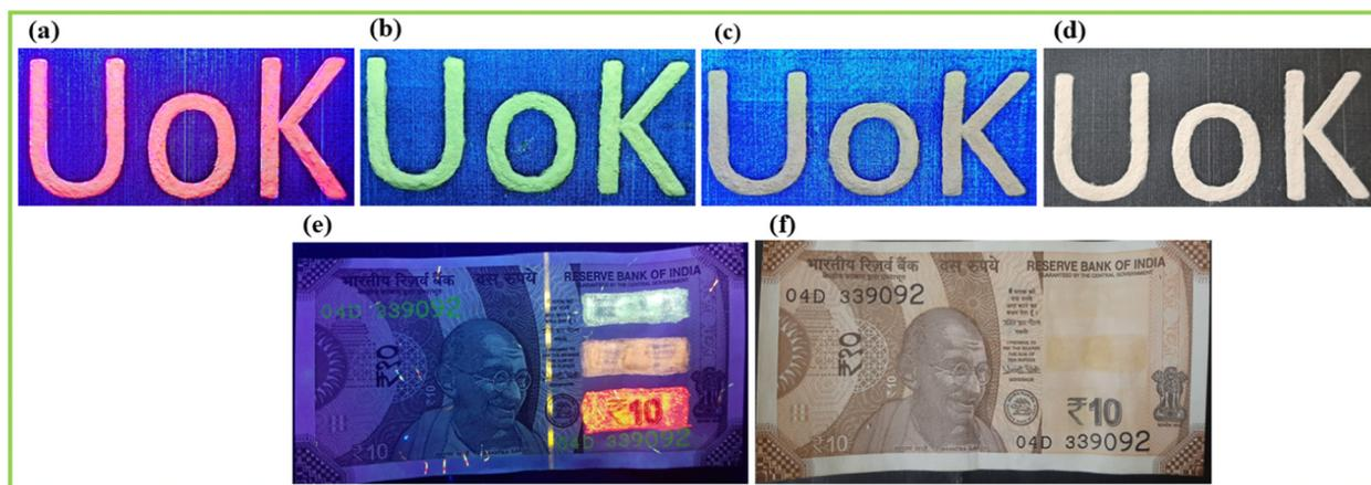
Fig. 16 Logo of the University of Kerala illuminated under UV radiation at 365 nm using security inks prepared using (a) SNMV:Eu<sup>3+</sup>, (b) SNMV, and (c) SNMV:Sm<sup>3+</sup> phosphors, and (d) under daylight, and (e) and (f) indicate the digital photographs of anti-counterfeiting labels marked on the Indian Rupee under 365 nm UV excitation (top to bottom-SNMV, SNMV:Sm<sup>3+</sup> and SNMV:Eu<sup>3+</sup> based inks) and daylight, respectively.
