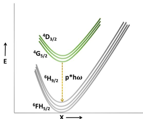
Fig. 9 Schematic model showing thermal quenching of  $Sm^{3+}$ .
