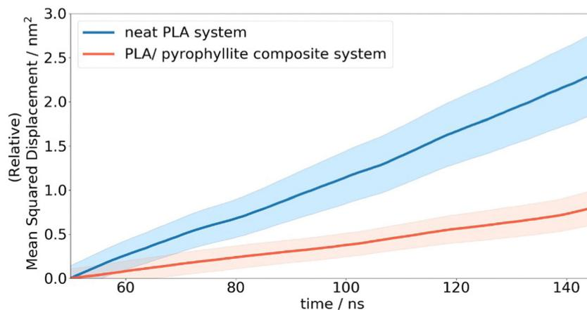
**Fig. 7** Average oxygen MSD plots in a neat PLA and PLA/clay composite slab system. Coloured regions depict the standard error associated with the mean squared displacement across 20 duplicate simulations.
