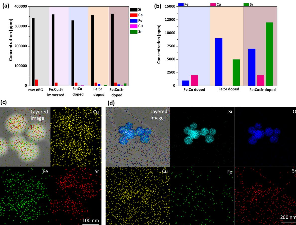
Fig. 3 Particle composition: SEM-EDX ensemble measurements of (a) all elements and (b) Fe, Cu, and Sr present in laser-doped samples. TEM-EDX elemental mapping of (c) Fe, Cu, Sr doped and (d) Fe, Cu, Sr immersed samples.
