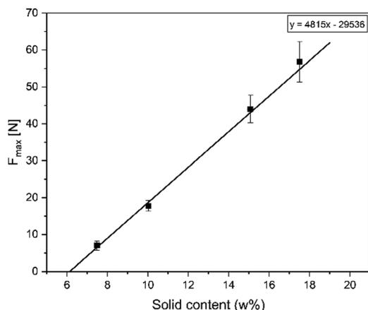
Fig. 5 Hydrogel stability depending on the solid content.
