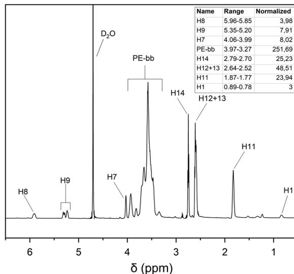
Fig. 3 <sup>1</sup>H NMR spectrum of hPG-NH<sub>2</sub> used for structural characterization.
