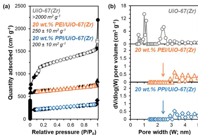
Fig. 3 (a) Adsorption–desorption isotherms (77 K) and (b) NLDFT pore size distributions from  $\text{N}_2$  physisorption for UiO-67(Zr) (grey circles), 20 wt% PEI/UiO-67(Zr) (orange triangles), and 20 wt% PPI/UiO-67(Zr) (blue diamonds). Isotherms for 20 wt% PEI/UiO-67(Zr) and 20 wt% PPI/UiO-67(Zr) are shifted vertically for clarity.
