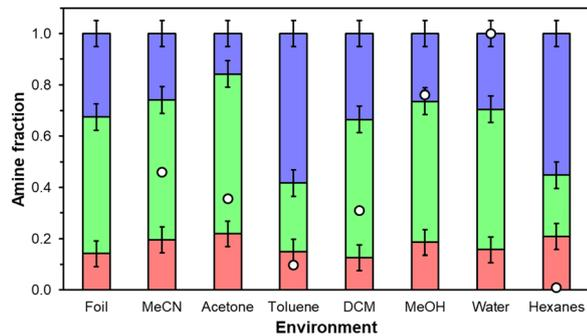
**Fig. 6** Primary (red), secondary (green), and tertiary (blue) amine distributions for as-synthesized poly(propylene imine) after exposure to different solvent environments of varying polarity (white circles) at ambient temperature (298 K) for 8 h. Distributions are determined *via*  $^1\text{H}$  NMR in  $\text{D}_2\text{O}$  solvent.
