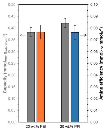
**Fig. 8** Amine efficiencies (orange, blue) and mass-normalized CO<sub>2</sub> capacities (grey) at 308 K for 20 wt% PEI/Uio-67(Zr) (orange) and 20 wt% PPI/Uio-67(Zr) (blue) from 40 mL min<sup>-1</sup> simulated air (400 ppm CO<sub>2</sub> in He) after 3 h under 40 mL min<sup>-1</sup> Ar at 383 K.
