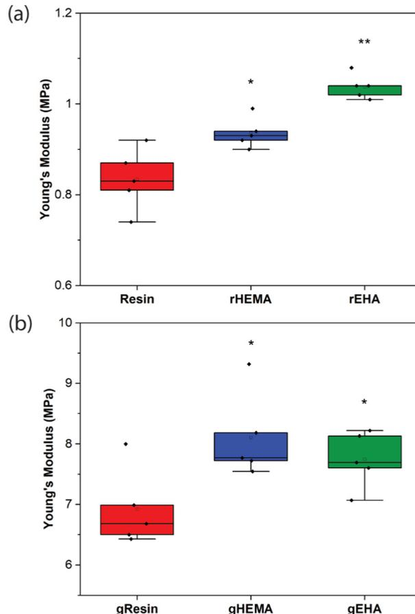
Fig. 3 Young's modulus values for (a) neat and (b) glass microsphere-filled samples. Individual data points as well as box and whisker plots are presented. \* indicates statistical differences from the control (either Resin or gResin). \*\* indicates statistical differences from all other conditions of the same type of sample (either neat or glass microsphere-filled).
