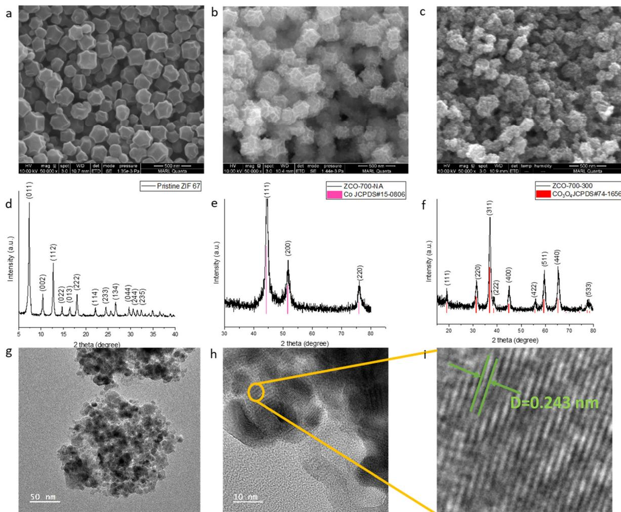
**Fig. 2** Characterization of the catalysts. SEM images and XRD patterns of the (a and d) as-synthesized ZIF-67, (b and e) ZCO-700-NA, and (c and f) ZCO-700-300. (g and h) TEM images of ZCO-700-300 at different magnifications. (i) A zoom-in image of h.
