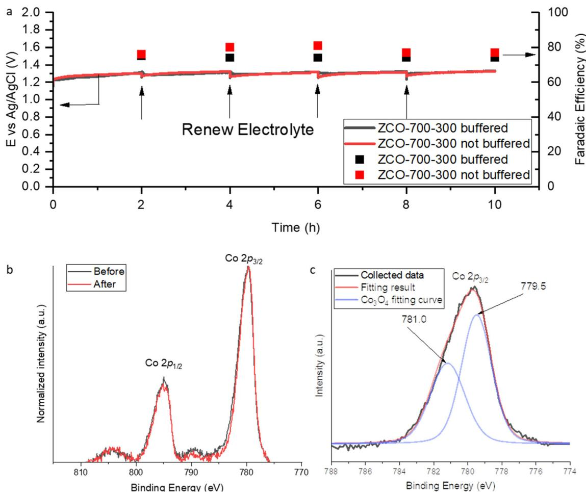
Fig. 4 (a) CP test results (90% IR compensated). (b) XPS results before and after the durability test. (c) Co<sub>3</sub>O<sub>4</sub> 2p<sub>3/2</sub> peak fitting curve.
