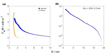
Fig. 5 Measurements of the normalised force between mica sheets as a function of separation, D, across 70 vol% EAN. (a) Linear scale forces at D < 10 nm with retraction (gold) shown from the innermost layer. (b) Log-linear representation of normal force displaying long-range decay with average decay length of  $\langle \lambda_s \rangle = 3.8 \pm 1.2$  nm.
