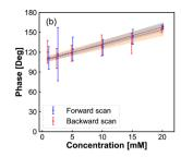
Fig. 4 Normalized optical amplitude (a) and phase (b) signals from lock-in amplifier vs.  $Fe(MeOH)_2$  concentration. DC potential scan from -200 mV to 300 mV with a scanning rate of 40 mV s<sup>-1</sup>, frequency of potential modulation is 75 Hz, the amplitude of potential modulation is 50 mV.
