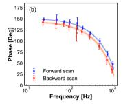
Fig. 5 Normalized optical amplitude (a) and phase (b) signals from lock-in amplifier with different frequency of potential modulation. DC potential scan from -200 mV to 300 mV with a scanning rate6 of 50 mV s<sup>-1</sup>, the amplitude of potential modulation is 50 mV, and the concentration of Fe(MeOH)<sub>2</sub> is 15 mM.
