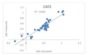
Fig. 5 Correlation plot of regioselectivity ( $\Delta\Delta E_{CAT2}$ ) predicted *versus* the experimentally obtained regioselectivity using the  $\Delta^{13}C$  shift and  $I_{C=C}$  stretch substrate parameters as indicated in eqn (2).
