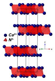
Fig. 2 Crystal model of  $Ca_2N$  showing Ca-N octahedrals. Electrons are thought to exist between the layers.<sup>17</sup>
