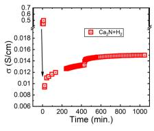
Fig. 4 EIS calculated conductivity from  $Ca_2N$  exposed to 5%  $H_2$  in Ar at 600 °C. The initial conductivity is for the  $Ca_2N$  phase, while the resulting conductivity is from  $Ca_2NH$  as shown by the post experiment XRD pattern 1 (see Fig. 1b).
