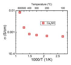
Fig. 6 Log of conductivity plot for the  $Ca_2NH$  system. A large jump in conductivity is observed between 400 and 500 °C. A similar jump was observed in the  $H^-$  conductor  $Ba_2NH$  by Altorfer et al.<sup>26</sup>
