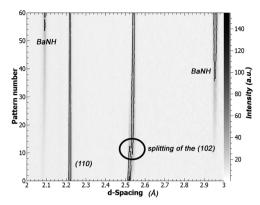
Fig. 8 Contour plot showing the evolution of NPD patterns *versus* pattern number (each pattern is  $\sim$ 2 min). After 20 min of exposure to N<sub>2</sub>, the (102) reflection of BaD<sub>2</sub> splits, while the (110) peak remains unchanged. The emergence of a second phase is clear at pattern number 40 (80 min).
