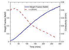
Fig. 10 Trend in calculated conductivity and phase fraction of BaND for doping of BaD<sub>2</sub> with  $N_2$  experimentally. The emergence of BaND is associated with a decrease in conductivity. Beyond 280 min, the resistance associated with the high frequency response increases dramatically making the accurate modelling of the  $R_s$  difficult.
