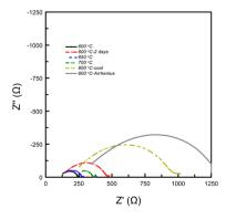
Fig. 5 EIS data collected on a  $Ca_2N$  pellet exposed to  $H_2$  gas at varying temperatures. Data is in chronological order. The data shows that the arc associated with a surface layer ( $10^{-9}$  to  $10^{-7}$   $F^{21}$ ) doubles after two days at 600 °C. The grey spectrum shows the data collected at 600 °C used for the conductivity log plot (see Fig. 6).
