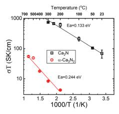
Fig. 3 Arrhenius plot of conductivity data measured on  $Ca_2N$  and  $\alpha$ - $Ca_3N_2$  systems.
