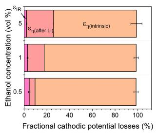
Fig. 4 A plot to show the fractional potential losses in the cathodic reaction for the lithium-mediated nitrogen reduction system due to overpotential and ohmic losses for a 0.6 M LiClO<sub>4</sub> in THF electrolyte with varying ethanol content. Fractional energy losses obtained using eqn (18) and (19).
