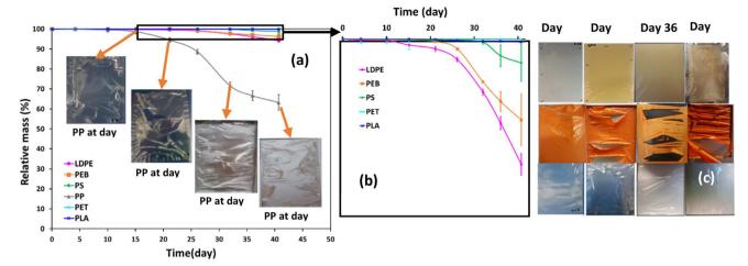
Fig. 1 Temporal mass loss for six selected polymers during accelerated weathering. Average quantities ± standard deviations were obtained by weighing each sample three times 24 h after removal from the weathering chamber (n = 3). The photos in (a) show PP at selected time intervals, while (b) magnifies data for all polymers except PP. The top, middle and bottom rows of photos in (c) show PS, PEB and LDPE respectively.
