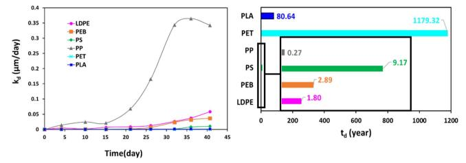
Fig. 5 Temporal changes in specific surface degradation rate (SSDR or  $k_{\rm d}$ , left) and the time required for total degradation ( $t_{\rm d}$ , right) for studied
