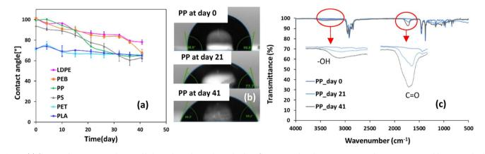
Fig. 3 (a) Changes in contact angle over 41 days of accelerated weathering. Contact angle values are expressed as average quantities  $\pm$  standard deviations from analysing three different subsamples for each sample (n=3), (b) photos of contact angle droplets produced by PP after days 0, 21 and 41 of the trial and (c) FTIR spectra for PP after the same time periods.
