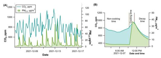
Fig. 9 (A) Cooking emission of indoor PM<sub>2.5</sub> and CO<sub>2</sub> measured by LCS during a 12 day period and (B) a one-day period from that 12 days, highlighting the differences between non-cooking time, cooking time, and decay rate.
