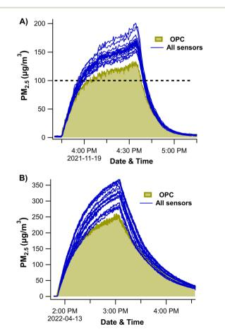
Fig. 2 SDS011 sensors and OPC measured PM<sub>2.5</sub> concentration for pre-campaign (A) and post-campaign calibration (B).
