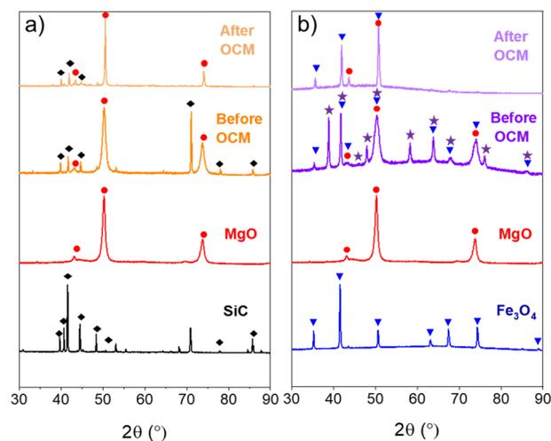
Fig. 3 X-ray diffraction patterns of a) SiC, MgO and SiC@MgO catalysts before and after OCM reaction under microwave heating (MW) and b) Fe<sub>3</sub>O<sub>4</sub>, MgO and Fe<sub>3</sub>O<sub>4</sub>@MgO catalysts before and after OCM under microwave heating (MW). SiC (◆), MgO (●), Fe<sub>3</sub>O<sub>4</sub> (▼) and Fe<sub>2</sub>O<sub>3</sub> (★).
