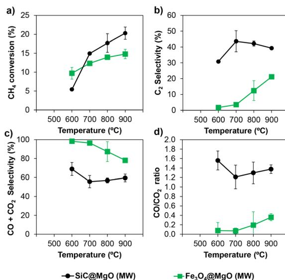
Fig. 7 a) CH<sub>4</sub> conversion, b) C<sub>2</sub> selectivity, c) CO + CO<sub>2</sub> selectivity and d) CO/CO<sub>2</sub> ratio for SiC@MgO and Fe<sub>3</sub>O<sub>4</sub>@MgO catalysts under microwave radiation (MW) conditions.
