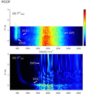
Fig. 15 2-D false-colour maps comparing the I<sup>3+</sup> ion velocities following 267 nm photolysis of CH<sub>3</sub>I and probing with (a) an 11.5 nm XUV pulse and (b) 805 nm SFI with  $I \sim 1300 \text{ TW cm}^{-2}$  (after subtraction of the NIR-only contribution), illustrating the very different relative weights of the DISS and DCE<sub>3</sub> signal contributions in the two cases. The relative intensities in both panels are depicted using the linear false-colour scale shown to the right
