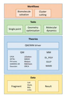
Fig. 1 Overview of ChemShell's modular framework. Chemical systems are defined by Fragment objects. Theories define QM, MM or QM/MM calculations on the Fragment data, which in turn can be invoked by highlevel chemical Tasks such as geometry optimisations. At the top level, Workflows are complex combinations of Tasks to support specific forms of modelling
